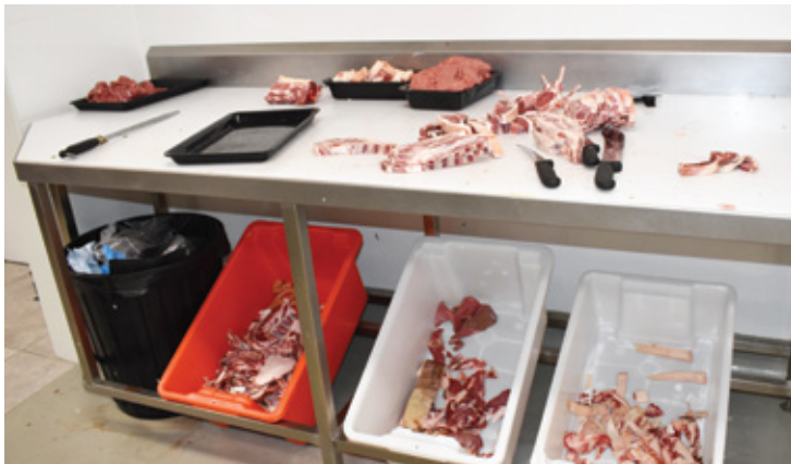
Custom-made boning bench with nally tub holders underneath.
